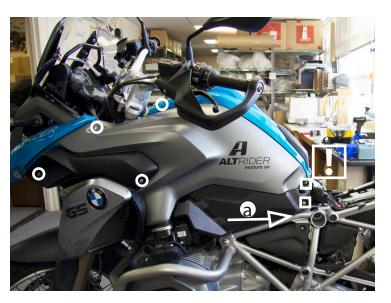
Switch to the left side and remove a total of (6) fairing screws using the T25 driver. Also remove trim piece (a) which is keyed and must slide backwards for removal. Fasteners represented as squares are long shoulder fasteners!
