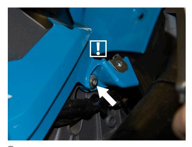
Carefully peel back fairing and remove the 2nd beak screw, this one is harder to get to and be careful not to scratch any painted plastic. This is a long shoulder fastener.
