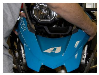
Spread the side of the beak and pull beak forward and away from bike. Note: the front of the beak is held in place by two locator pins.
