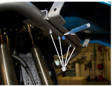
Hold your upper bars in place while you start threading the (4) M6 x 35 mm fasteners and washers. Add thread locker to each fastener, do not tighten all the way.
